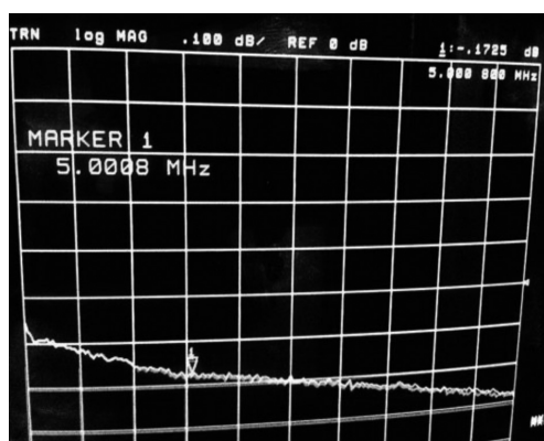
Figure 12 – Insertion loss caused by the balun
