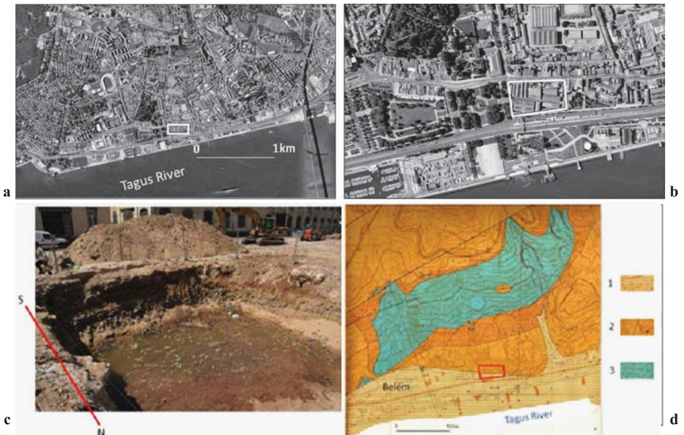
Fig. 1 – The studied area of Belém (Lisbon), near the Tagus River, (a) and (b) before the beginning of the urban renewal and view of one of the ditches in July 2008 (c) . Geological map (d) , where 1 – “LVC” cover by landfill (Upper Holocene), 2 – “Lisbon Volcanic Complex” (LVC) (Neocretaceous), 3 – Limestones (Upper Cenomanian), Moitinho de Almeida (1986).
