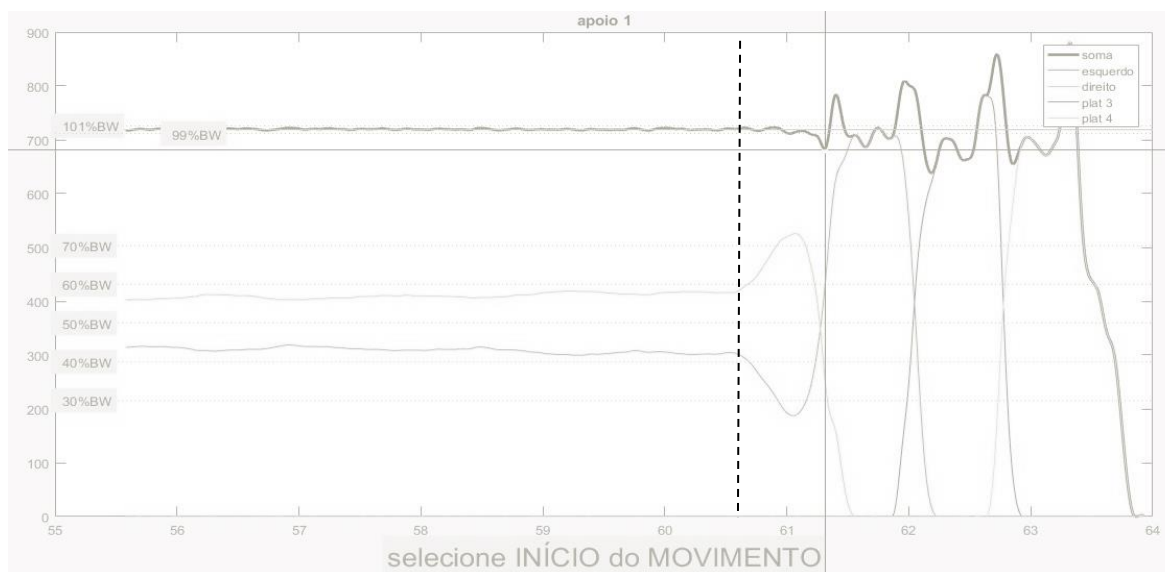
Figure 2: Indication of the beginning of the weight transfer (---) and the beginning of the movement (—).
