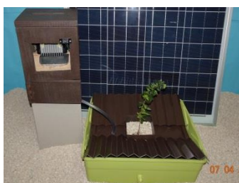
Figure 5 – Irrigation system for plants and trees that take the water from humidity of the air.
