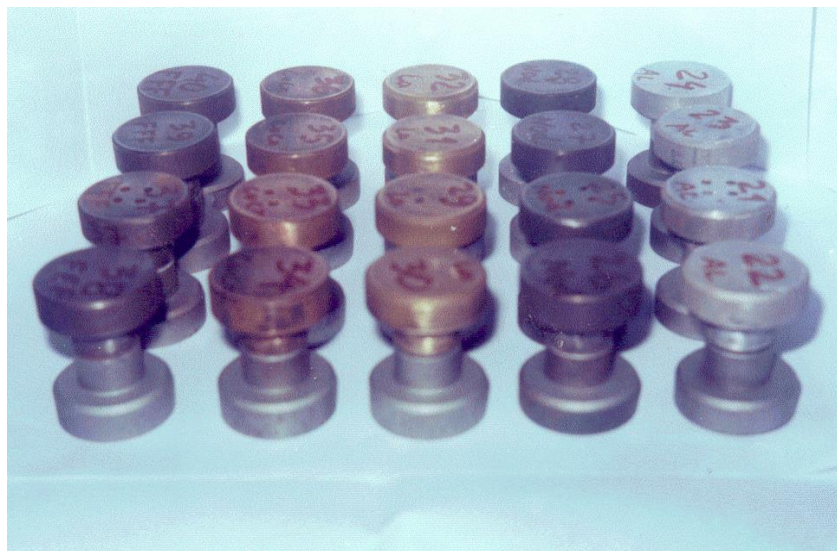
Figure 5 - Agglutinated assemblies of coated specimens with against-specimens (specimens on top)
