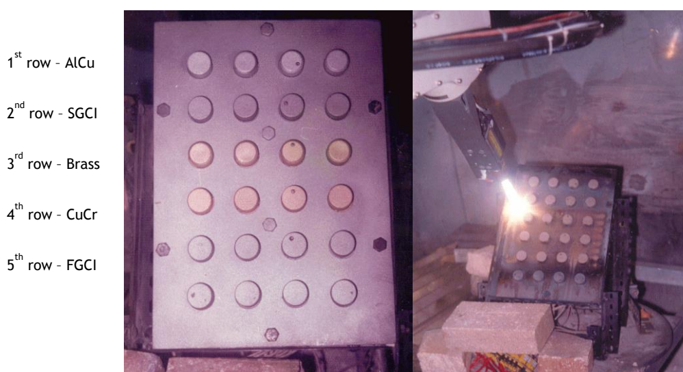
Figure 3 - Specimen's assembly in the spraying plate (on the left) and robotic spraying of the bond coating with a spray angle of 90° (on the right)
