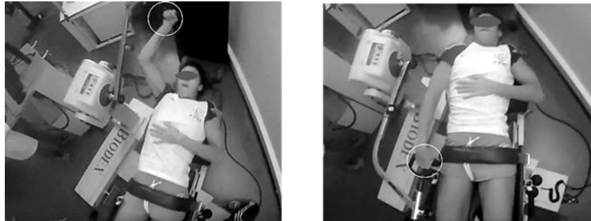
Figure 1. Conditioning in Biodex for upper limb simulated action (left: initial position; right: final position). The identified circles represent the hand positioning.
