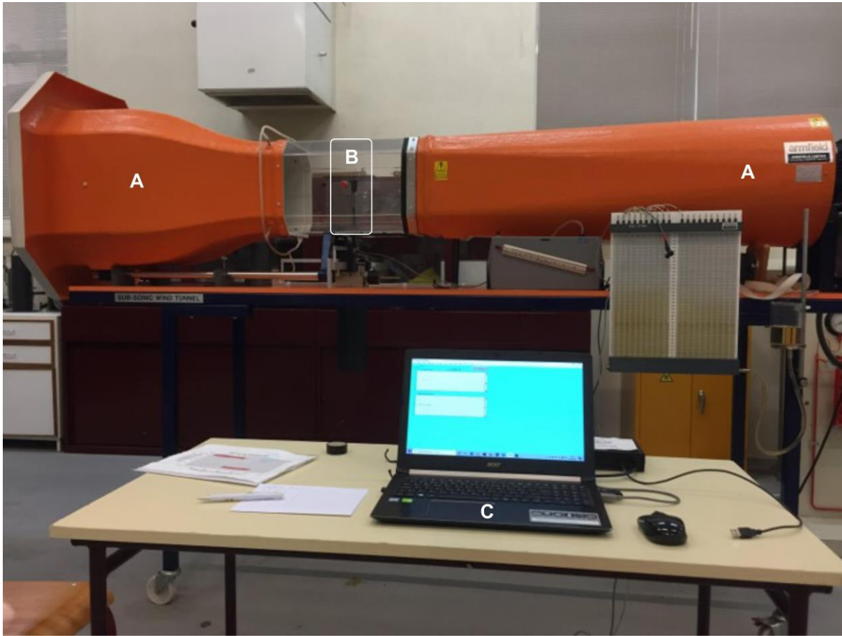
Figure 1. The assessment setup with the Wind Tunnel (A), Type A sensor (B) and Aquanex system (C).
