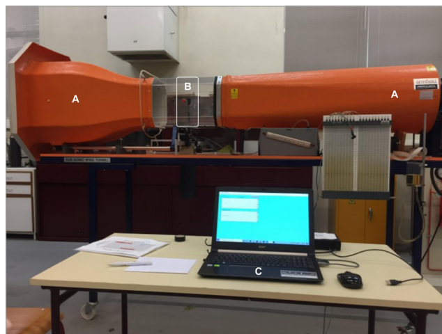
Figure 1. The assessment setup with the (A) Wind Tunnel, (B) Type A sensor and (C) Aquanex system.
