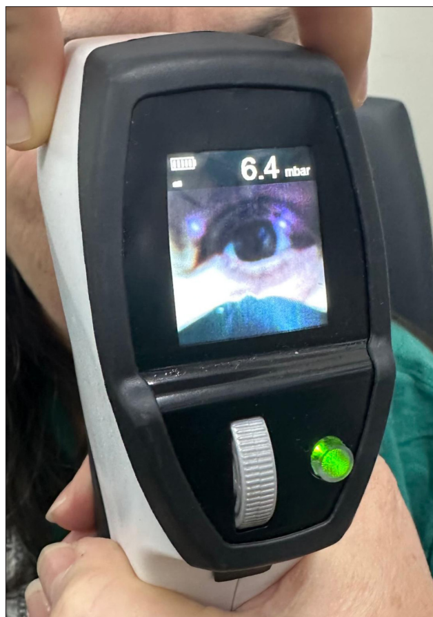
Figure 2. The Brill corneal esthesiometer in clinical use. The device is positioned in front of the patient's eye, and the integrated digital display shows real-time visualization of the ocular surface, stimulus pressure (6.4 mbar), and battery status. The ergonomic design enables single-handed operation, with a control dial for stimulus adjustment and a colored indicator light signaling device readiness. The system delivers non-contact air pulses to the cornea and uses a camera coupled with infrared LEDs for optimal alignment and precise distance control, ensuring standardization and reproducibility during corneal sensitivity assessment in both clinical and research settings.
