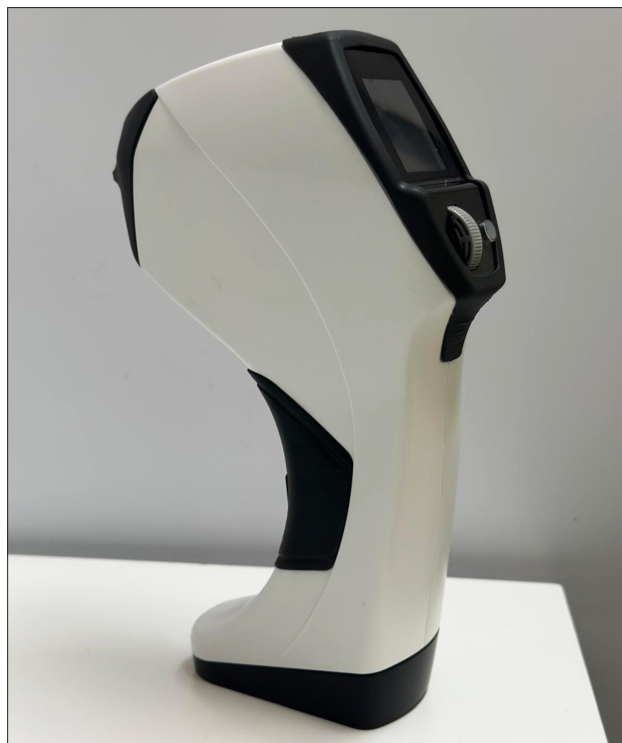
Figure 1. The Brill corneal esthesiometer is a portable, handheld, and non-contact device engineered for precise measurement of corneal sensitivity. Its structure features an ergonomic handle, a digital display for real-time stimulus adjustments, and an electronic positioning system that includes a camera and dual infrared LEDs for accurate alignment and distance control. The device employs a nozzle to deliver controlled pulses of air to the cornea and can be used either as a standalone handheld unit or mounted on a slit lamp. It offers five selectable pressure levels, an integrated sensor to record delivered stimulus, and operates with rechargeable battery power—streamlining assessments of corneal nerve function in both clinical and research contexts.
