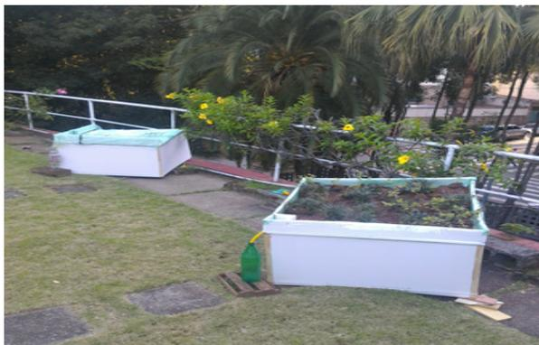
**Illustration 1** – Prototypes with and without green roof
