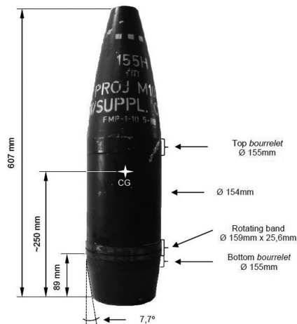
Figure 3 - M107 HE Grenade principal external dimensions.
