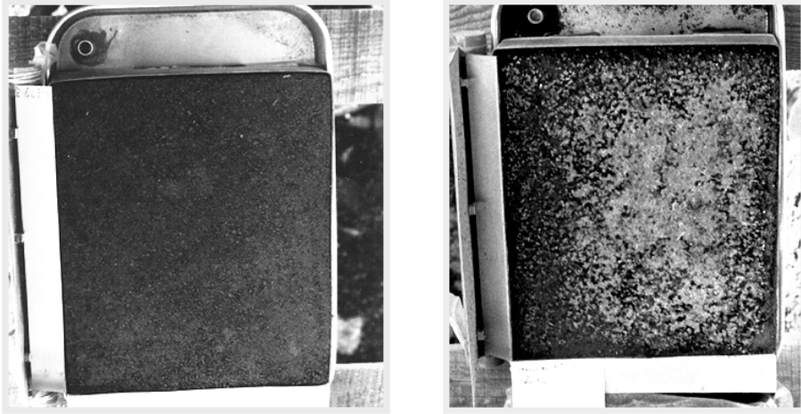
Figure 3 – Soil surface at the beginning of the experiment (left) and after 90 mm precipitation (right), for bare soil treatment (note the crusted surface)
