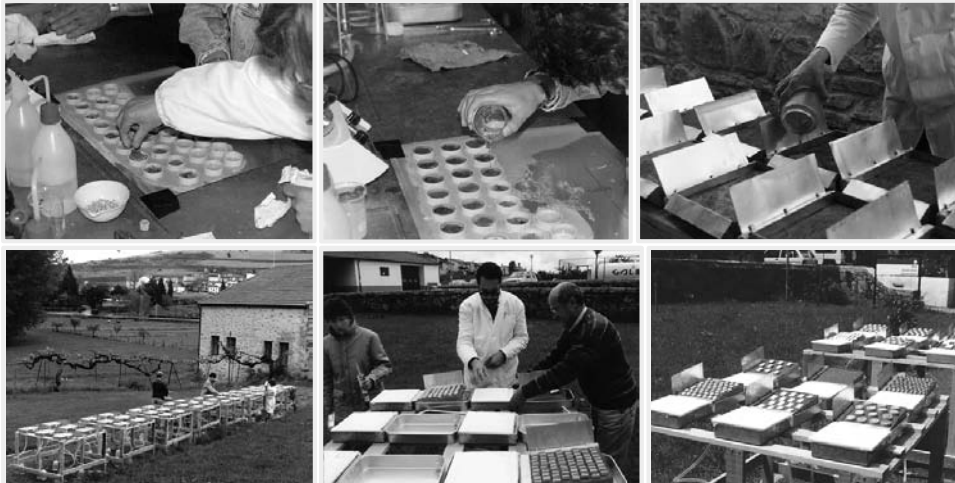
Figure 1 – Experiment preparation and installation: top – preparing circular simulated rock fragments (lead pieces and melted paraffin) and filling soil boxes (boards are splash collectors); down – installing boxes outdoor (containers on the ground are infiltration collectors, boxes with cover plates are runoff / wash collectors)
