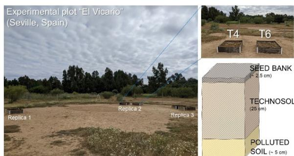
**Figure 1** - Experimental plot and scheme of the rehabilitation system based on Technosols.
