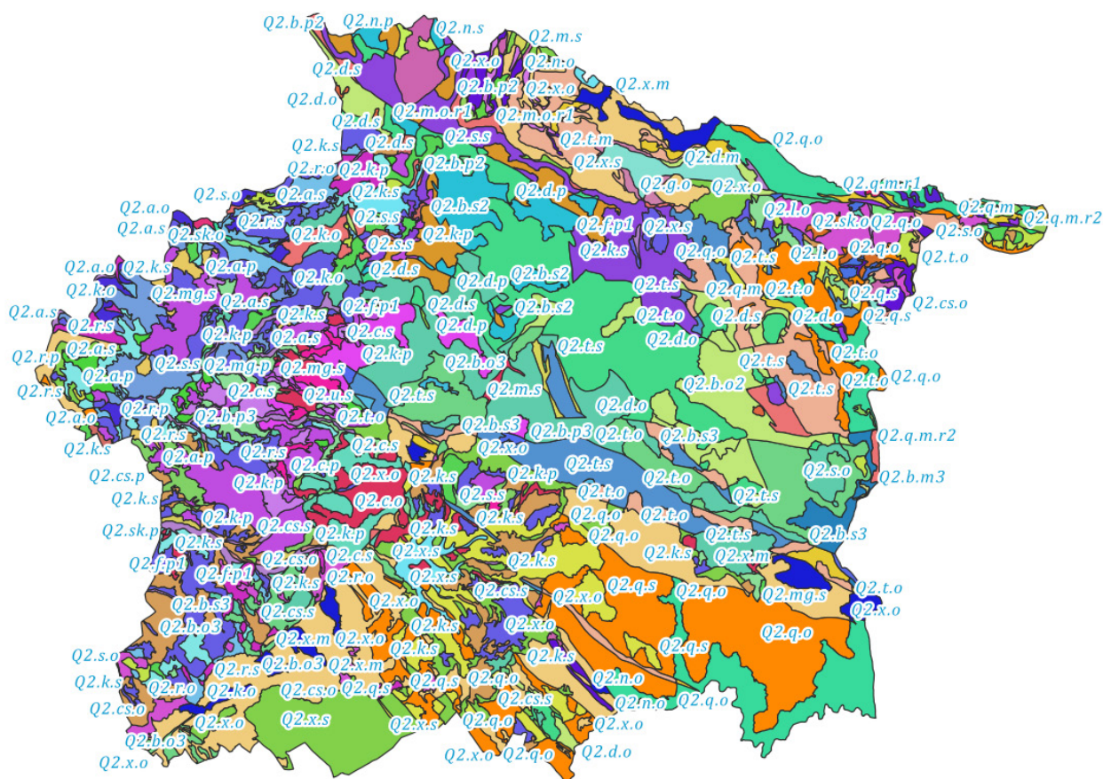
Figure 2 - Definitive homogeneous units of Beja test area. Each colour corresponds to a specific homogeneous unit, which is defined by a combination of different symbols (specified in the text): climate, lithological material, relief and rocky outcrops abundance (if not “o”).
