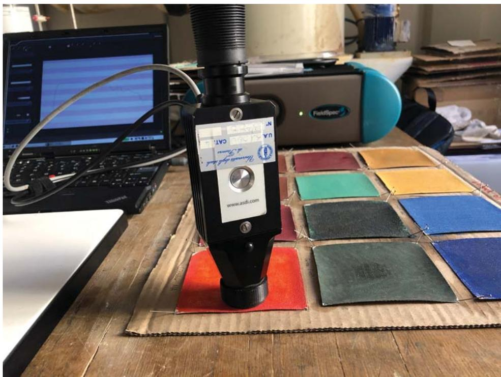
**Figure 1** - Portable hyperspectral sensor, ASD FieldSpec FR Pro 3.
