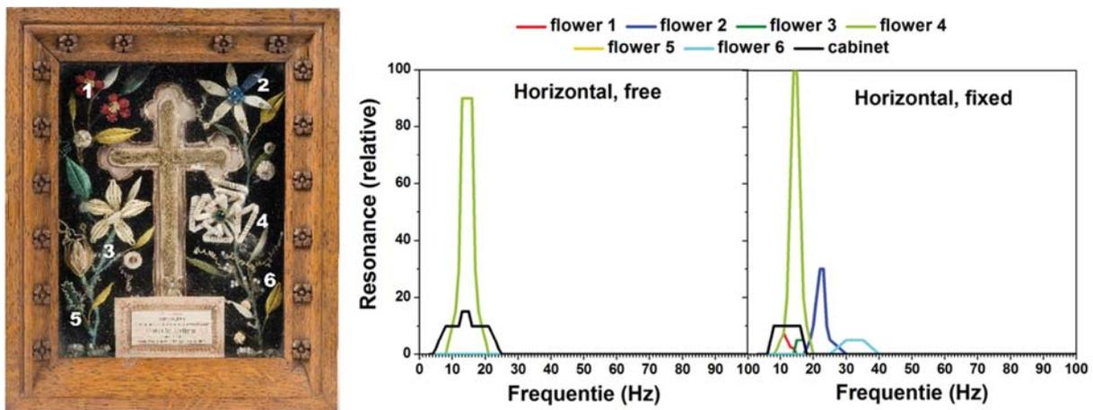
**Figure 4** - Left: Original mixed-media object inspired on the Enclosed Gardens with the indication of the flower numbers used in the graphs (©KIKIRPA, Brussels, x109633). Right: Resonant frequencies for different flowers and the cabinet itself, for horizontal vibrations and for a free and fixed position of the cabinet on the shaker table.
