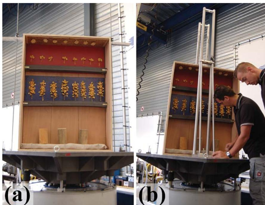
**Figure 2** - Model of Enclosed Garden mounted on a vibration table at Sebert Trillingstechniek B.V. (a) Fixed simulating transport; (b) Free-standing simulating exhibition. The rod structure prevents the model from “wandering”.
