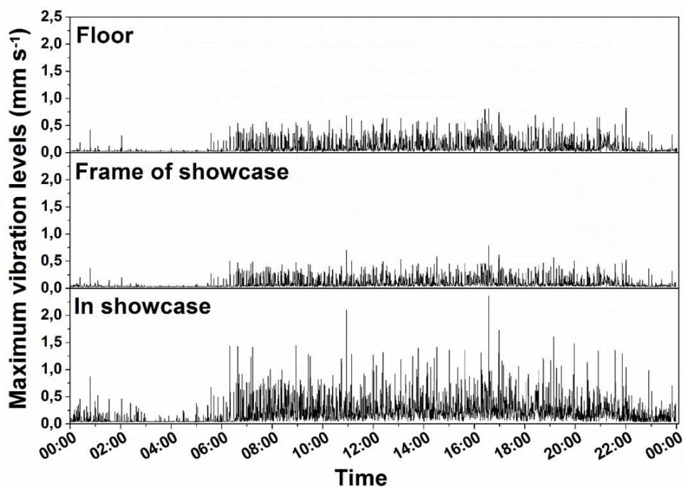
**Figure 7** - Maximum vibration levels measured for every thirty seconds during the 24 hours monitoring period; overview for the three measuring locations: floor, frame of showcase, and in the showcase next to an Enclosed Garden.
