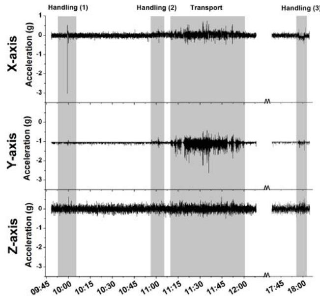
**Figure 5** - Shocks and vibrations measured during handling and transport of an original Enclosed Garden to a temporary exhibition. X-axis: driving direction of the truck; Y-axis: vertical movement; Z-axis: lateral movement.
